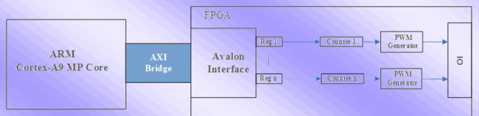
Figure 3: The fast pulse generation circuit hardware.
