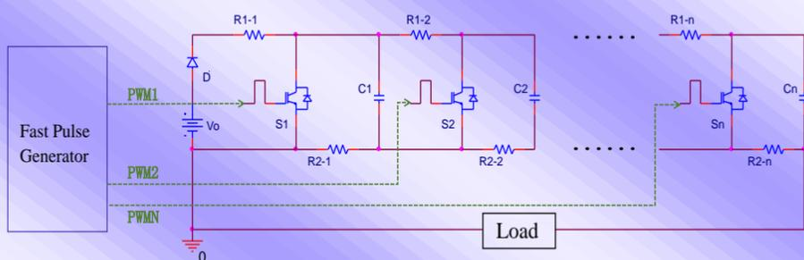
Figure 1 The schematic of the solid-state PFN-Marx generator.
