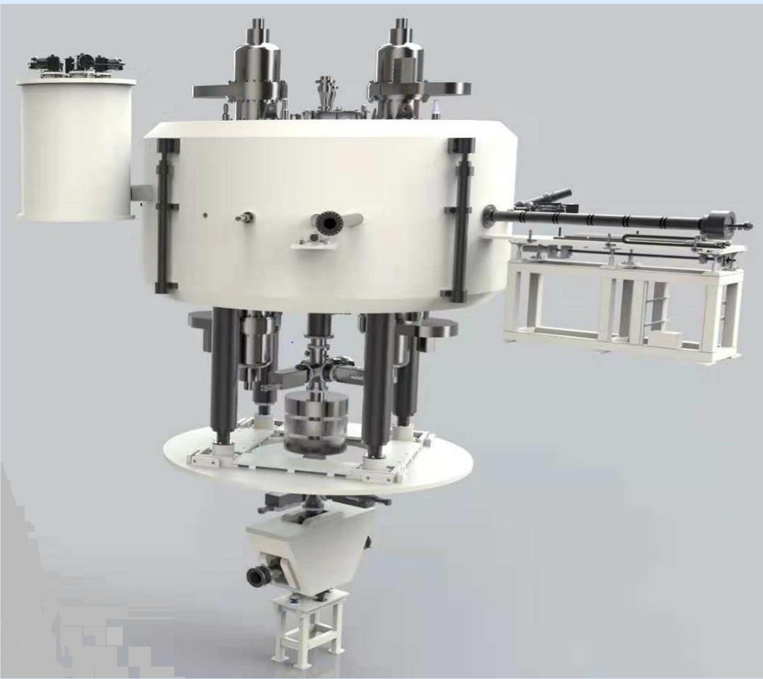
Fig.1 The cyclotron structural model
