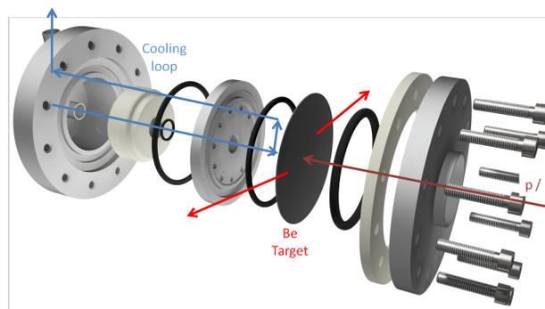
Figure 6: Target design for a NOVA ERA source at a power level of 0.4 kW.
