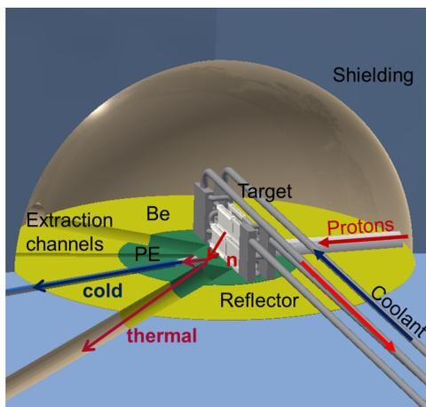
Figure 4: The target / moderator / shielding assembly.
