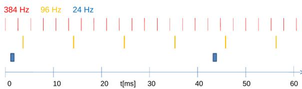
Figure 2: Pulse structure provided by the accelerator for the large scale facility.
