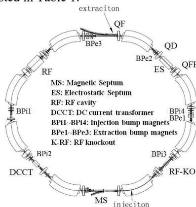
Figure 1: Schematic layout of the HIMM synchrotron ring.
