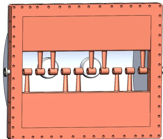
Figure 3: The inner structure of proposed HOM-DTL.
