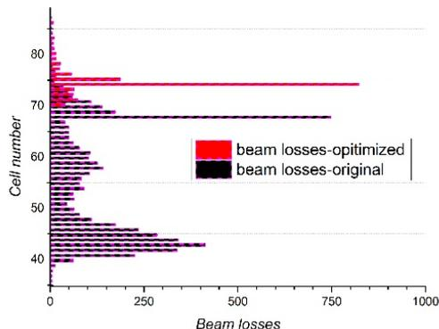
Figure 4: Beam losses of original and optimized designs.
