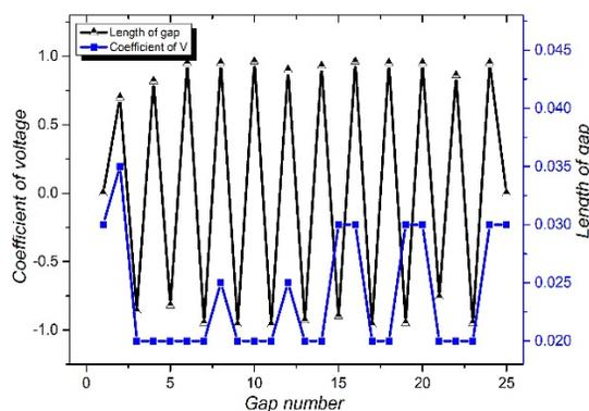
Figure 6: The voltage and length of gap in each cell.
