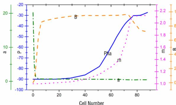
Figure 2: The optimized parameters in RFQ section.
