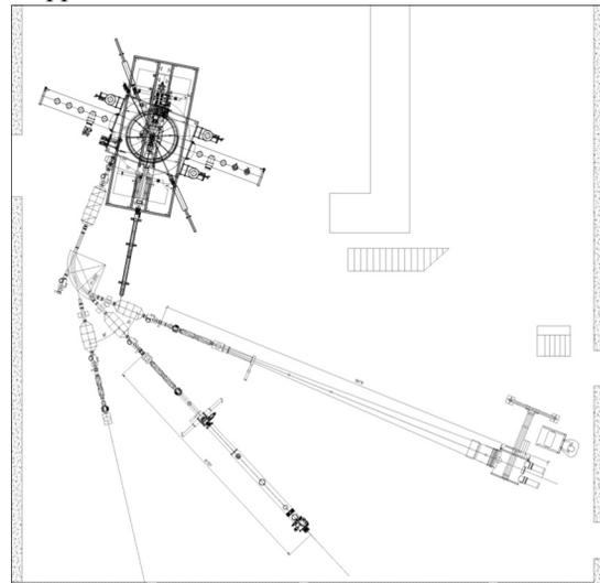
Figure 6: Scheme of experimental beam lines. From left to right: RP line; SEE testing line; TM line
