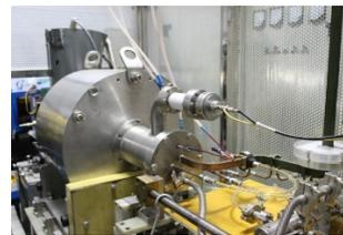
Figure 4: LAPECR2 ion source on a test bench.
