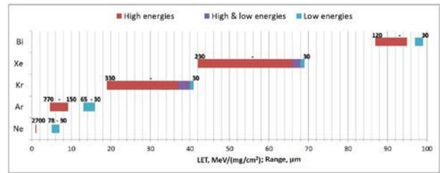
Figure 11: Quasi-continuous LET spectrum at the high-energy facility using degraders – LET & Range for different type of ions.
