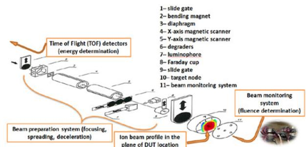
Figure 2: Beam transfer channel layout.
