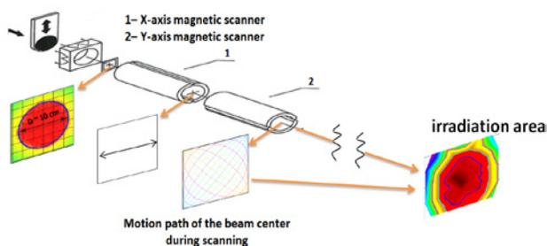
Figure 3: Beam modification system.
