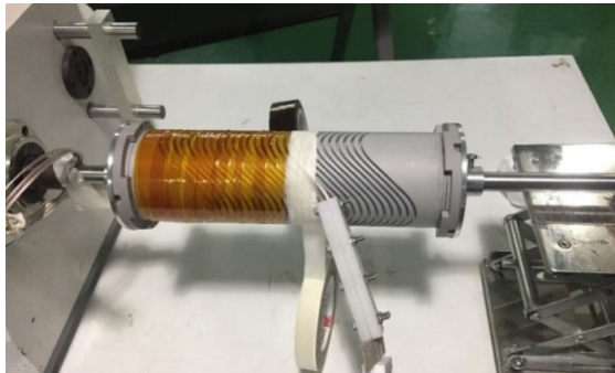
Figure 12: Winding process of the subscale quadrupole coil.
