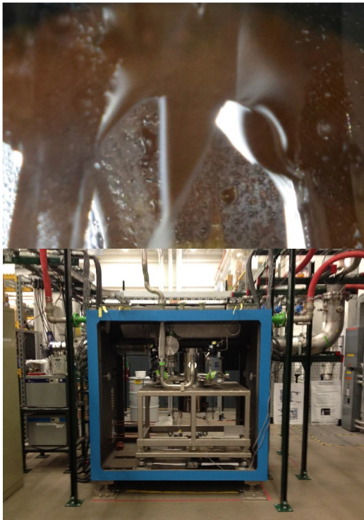
Figure 9: Liquid lithium charge stripper module (bottom) and the established lithium film (top).
