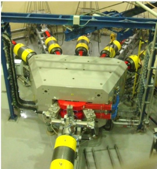
Figure 7: Beam transport channels, where: 1- \pm 50^\circ bending magnet, 2- quadrupole lenses.
