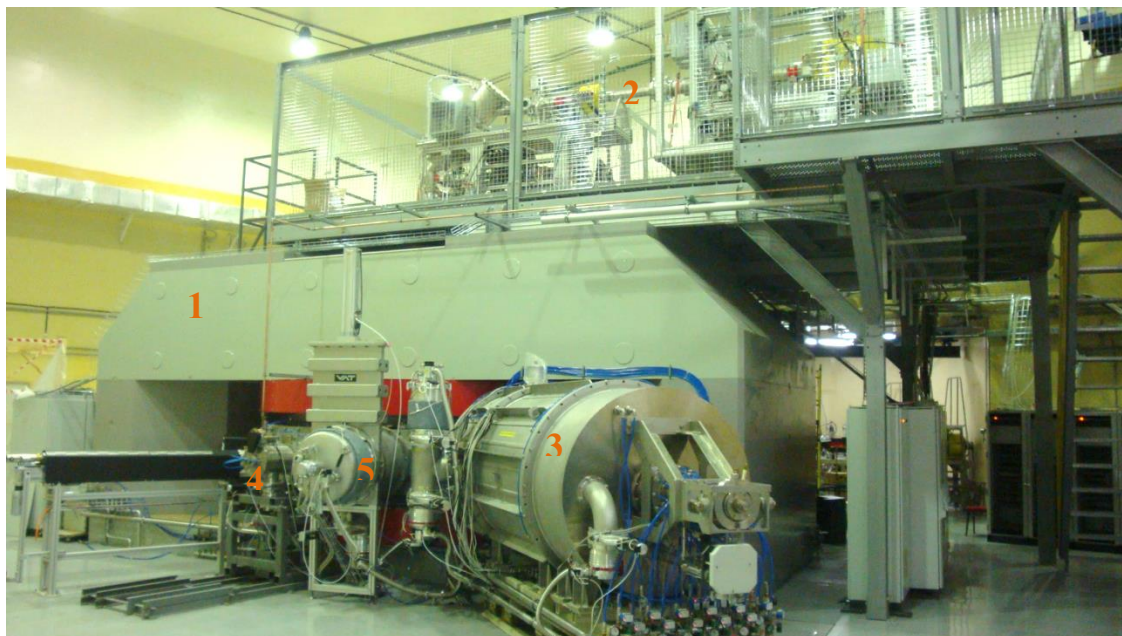
Figure 4: The new DC-280 cyclotron, where: 1- Main magnet, 2- HV injection system, 3- RF resonator, 4- Flat-top resonator, 5-Vacuum pumps.
