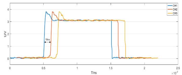
Figure 4: The multi-channel fast pulse output signals.
