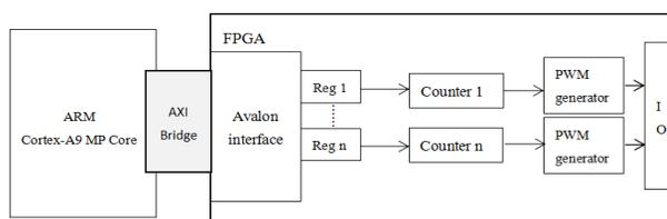
Figure 3: The fast pulse generator hardware structure.
