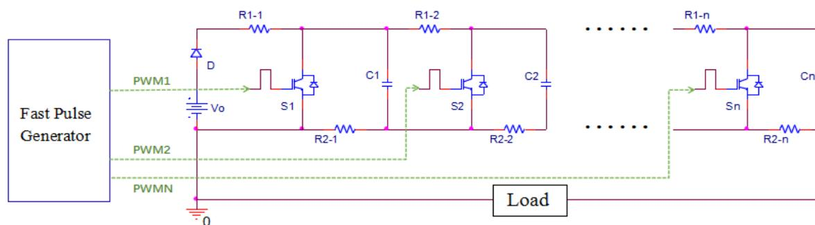
Figure 1: The schematic of the solid-state PFN-Marx generator.
