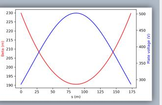
1.  $n\pi$  phase advance over T-insert region. 2. Equal beta function in drift region  $\beta_x = \beta_y$ . 3. Octupole applied in drift region and strength scales with  $1/\beta(s)^3$ .
