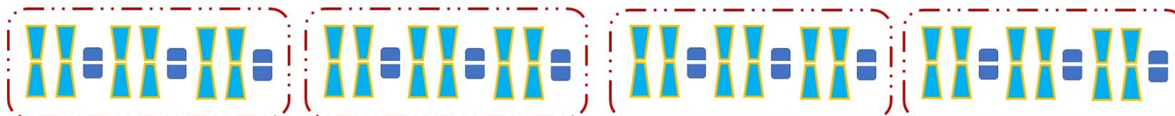
4 CRYOMODULES X [6 X 162.5MHz HWR + 3xSC-Solenoids]
