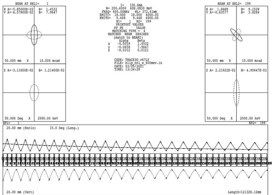
200 MeV beam drifting through CCL
