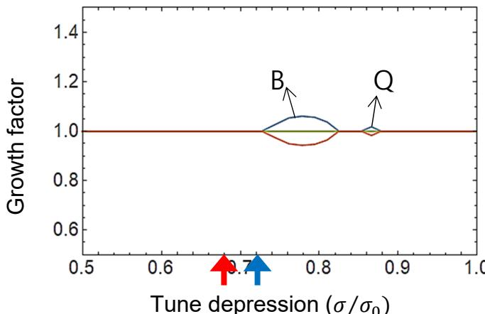
The 4<sup>th</sup> order particle resonance stop band is wider than the envelope instability stopband.
