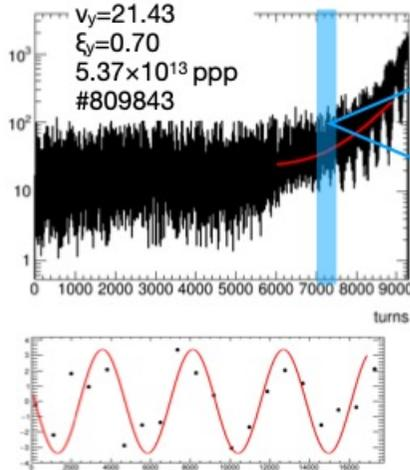
Oscillation of coupled bunch mode of resistive wall effect was observed ( $\mu=2$ )
