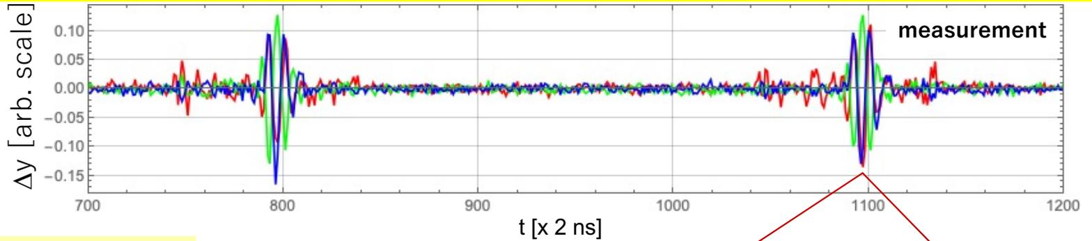
**Measurement suggests stable and unstable points along the bunch caused by the processing clock**
