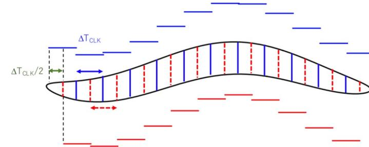
The timing of two systems is  $\Delta T_{CLK}/2$  shifted.
