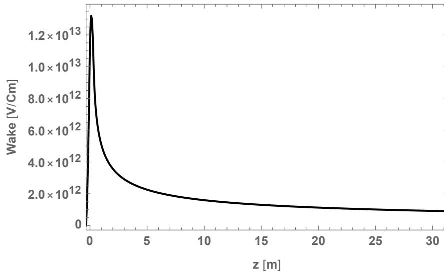
Resistive wall wake potential of the SUS316L vacuum duct, modeled with a cylindrical pipe of inner diameter 160 mm, thickness 2 mm, and length 1567.5 m.
