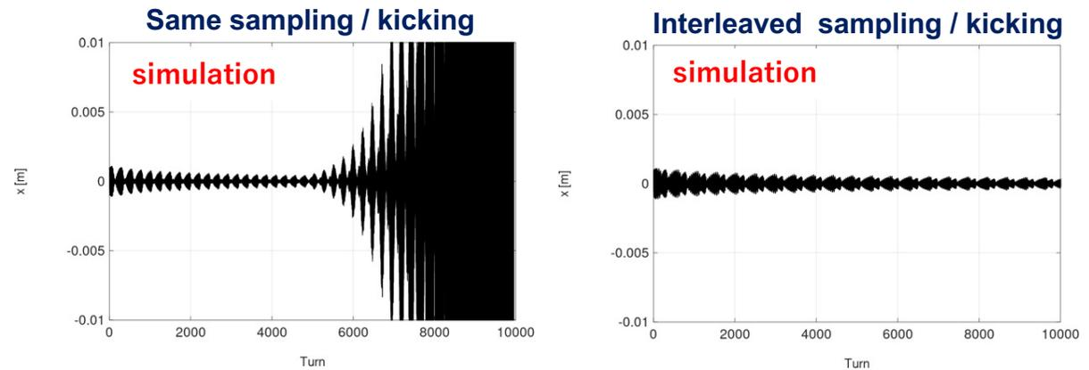
Simulated results w/o and with the time interleaved sampling and kicking by two feedback system.
