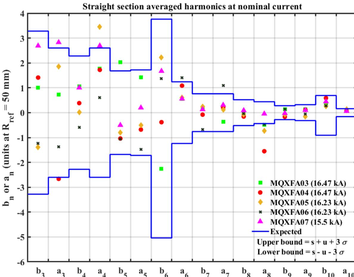
Integral harmonics to be measured in Coldmass
