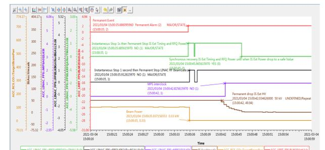
Fig. 7: Diagram of permanent protection for RCS BLM
