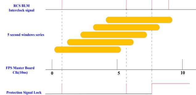
Fig. 5: Diagram of RCS BLM processing
