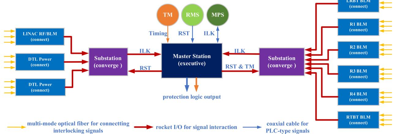
Fig. 4: Layout of CSNS fast machine protection system.
