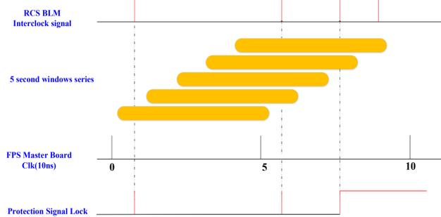
Fig. 5: Diagram of RCS BLM processing
