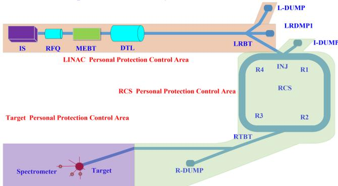
Fig 2: Schematic diagram of beam target and control area.
