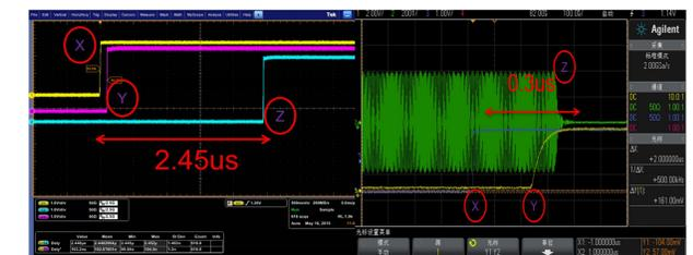
Fig. 8: Response time test for FPS.
