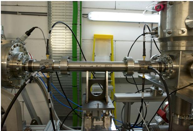
Figure 4: Setup for ToF measurement between two BPM.
