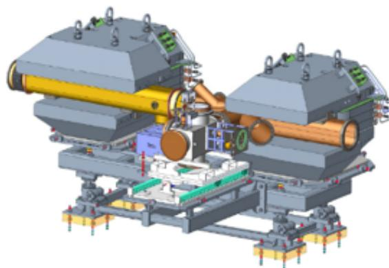
Figure 4: New ring injection chicane design.
