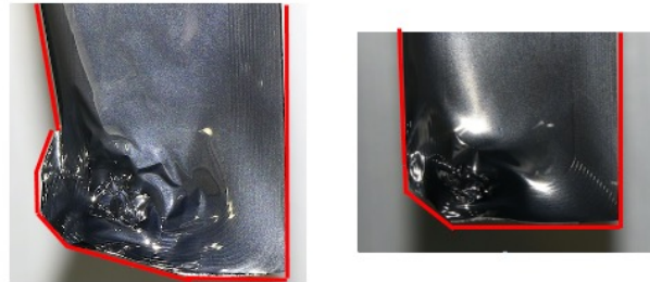
Figure 5: Two foils after conditioning demonstrating the unpredictable deformation.
