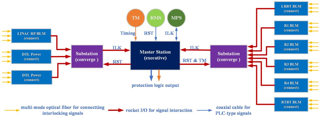
Figure 4: The schematic diagram of signal link.
