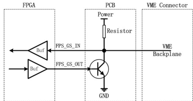
Figure 6: The schematic diagram of logic "OR".
