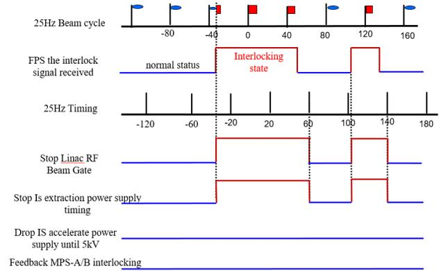
Figure 10: The schematic diagram for instantaneous protection logic.
