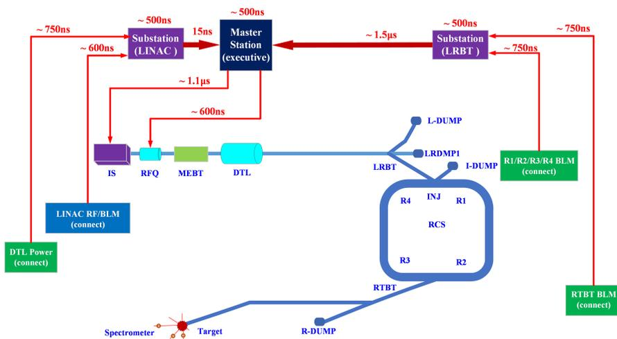
Figure 12: The response time of critical link.
