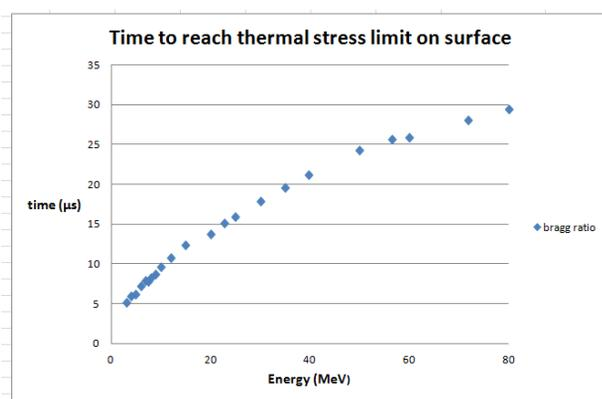
Figure 1: The relationship between the thermal stress limit in the material (copper) and the cumulative beam loss time. ①  $I=15$  mA,  $\sigma_x = \sigma_y = 0.2$  cm,  $J=62$  J/gm (energy density); ② Un-chopped beam, 15 mA; ③ Beam size: 0.2 cm  $\times$  0.1 cm RMS; ④ Hitting the components directly.
