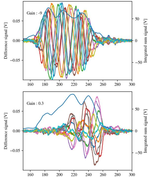
Figure 7: Instability snap-shot taken at three different intensities. The difference signal is proportional to position and intensity. The integrated sum signal shows the longitudinal profile. As the intensity and space charge is increased, huge amplification is observed from the head to the tail.
