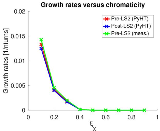
Figure 7: Growth rates as function of the horizontal chromaticity of the instability for a bunch intensity of  $2.0 \times 10^{11}$  ppb. Pre-LS2 and post-LS2 cases have been computed with PyHEADTAIL simulations and compared with the measured values obtained with optimized damper settings.
