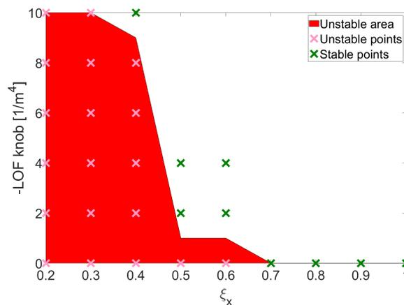
Figure 9: Stability map at injection energy for the nominal LIU beam ( $4 \times 72$  bunches with  $N=2.6 \times 10^{11}$  ppb). Stable points are represented in green and unstable points in magenta. Using these points the unstable area is depicted in red. A simulation point is considered to be stable if over 10000 SPS turns there is no exponential amplitude growth, emittance blow-up is below 10% and losses are below 1%.
