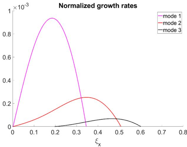
Figure 5: Normalized horizontal instability growth rates as function of the horizontal chromaticity of the head-tail mode 1 in magenta, mode 2 in red and mode 3 in black. The growth rates have been computed by using the Sacherer theory with Gaussian bunches for the SPS impedance model at injection energy for the Q20 optics.
