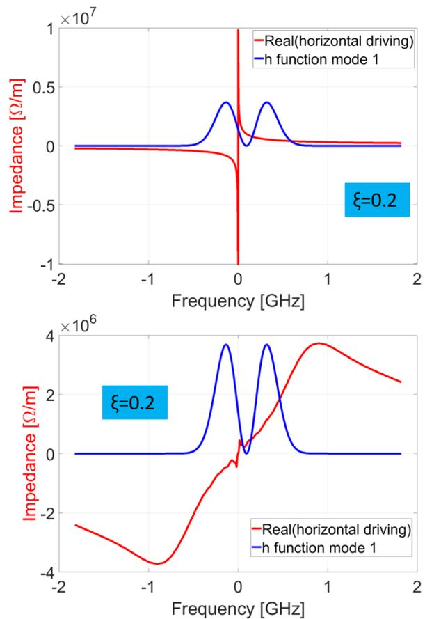
Figure 4: Power spectral density for the mode  $l = 1$  in arbitrary units for a chromaticity  $\xi = 0.2$  (blue) together with the SPS wall impedance model (top) and the SPS kickers without serigraphy (bottom) at injection energy for the Q20 optics.
