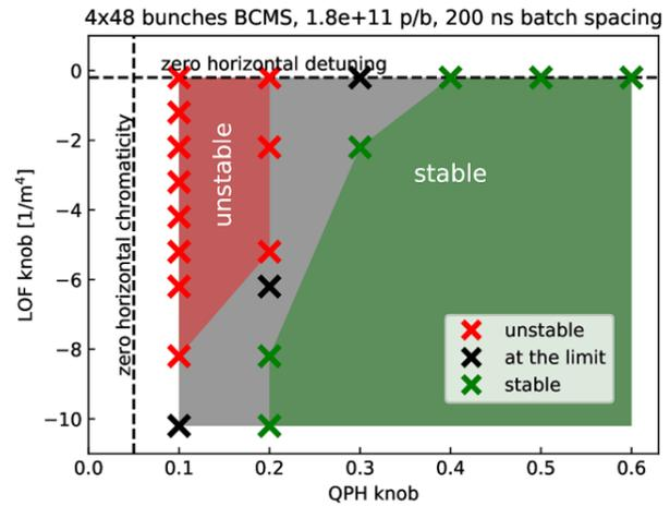
Figure 2: Measured horizontal beam stability for different chromaticity and octupole settings, where the QPH knob controls the normalised horizontal chromaticity  $\xi_H$  and the LOF knob controls the normalised octupole strength. The values for zero chromaticity and no amplitude detuning are indicated by dashed lines. The markers indicate unstable (red), stable (green) and settings where some shots were stable and some unstable (black) as obtained from about 5 shots per setting.
