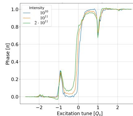
Figure 5: Examples of BTF phases obtained numerically for a chromaticity of 6 units,  $a\epsilon_x = 10^{-4}$  and including wakefields. The excitation tune is shifted to the betatron tune and expressed in units of the synchrotron frequency.
