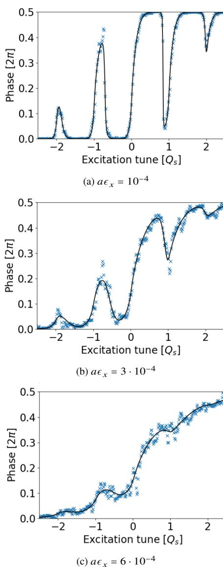
Figure 4: Examples of BTF phases obtained numerically (blue crosses) and the corresponding fit (black lines) for a chromaticity of 15 units and different detunings. The excitation tune is shifted to the betatron tune and expressed in units of the synchrotron tune.
