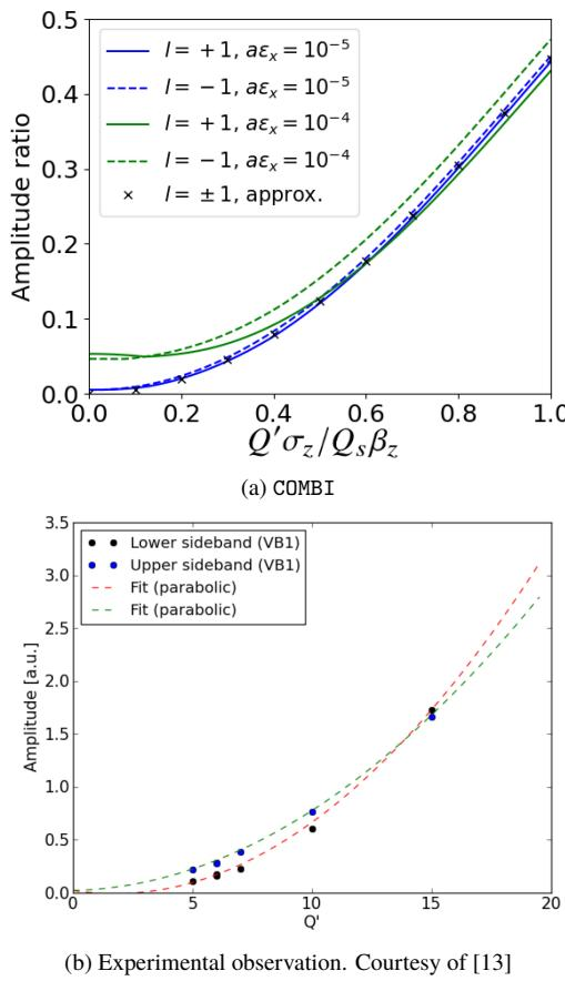
Figure 2: Amplitude ratio obtained analytically (upper plot, black crosses) and numerically for different sidebands  $l$  and detuning. The datasets are labelled by their r.m.s. detuning driven by the direct term  $a\epsilon_x$ .  $\epsilon_x$  is the geometric transverse emittance. The lower plot shows the result of an experiment at the LHC (dots). Parabolic fits were tried whereas the theory rather suggests Eq. (7).
