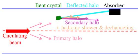
Figure 2: Schematic representation of the working principle of a crystal-based collimation system [6].
