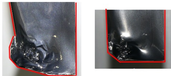
Figure 5: Two foils after conditioning demonstrating the unpredictable deformation.
