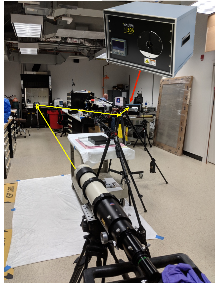
Calibrating the pyrometer in the foil lab
