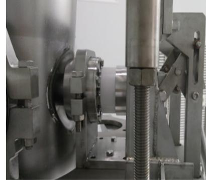
$Q_e$  adjustable, four orders of magnitude. Antenna moving range:  $\pm 20\text{mm}$ . HWR vetical test
