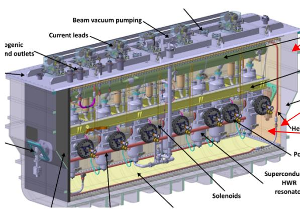
→ Isolation vacuum : pumped airtight tank
