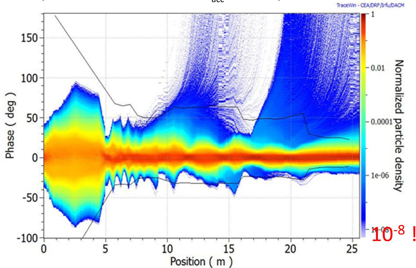
Longitudinal beam « probability » profile (cavities tuned with BPM &  $\pm 1\%/\pm 1^\circ$  tuning errors)
