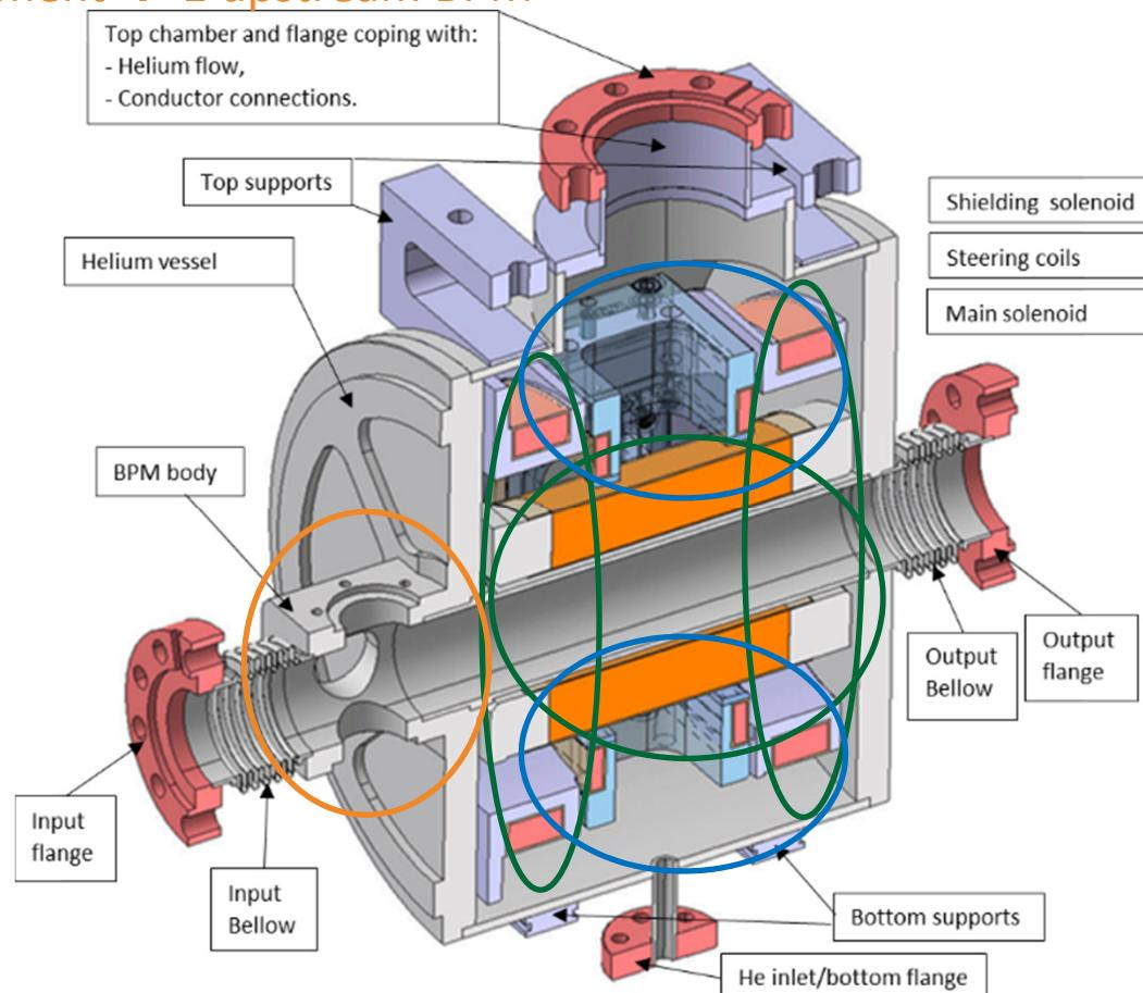
SP are tuned (focusing/steering) to keep the beam matched (between CM) and on axis (BPM)
