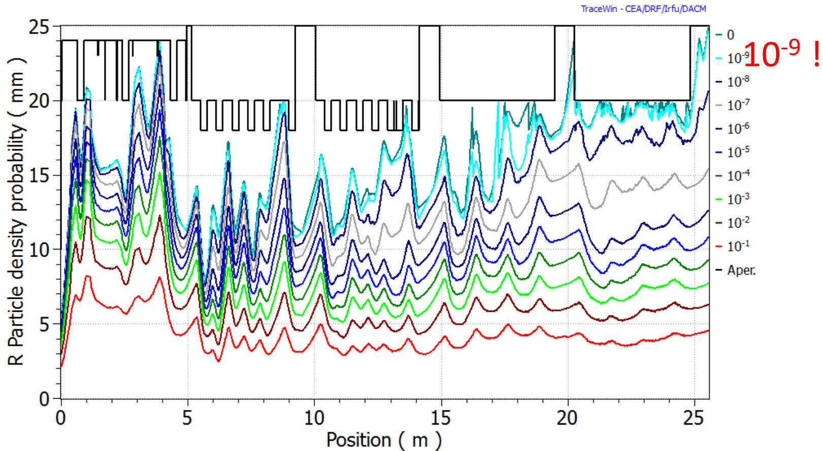
Transverse beam « probability » contour plots (steerer with BPM &  $\pm 2$  mm position errors)
