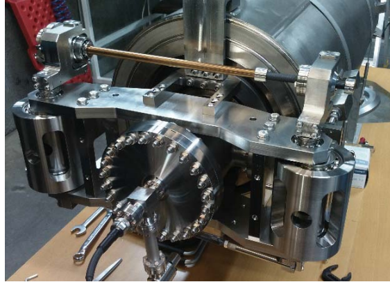
Assembly and adjustment of the cold tuning systems
