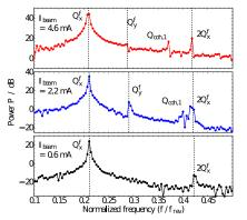
Figure 6: Shift of coherent quadrupole mode Q<sub>coh,1</sub> with beam current.
