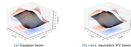
Figure: Electric fields in r.m.s. equivalent distributions with same  $\sigma_{x,y}$
