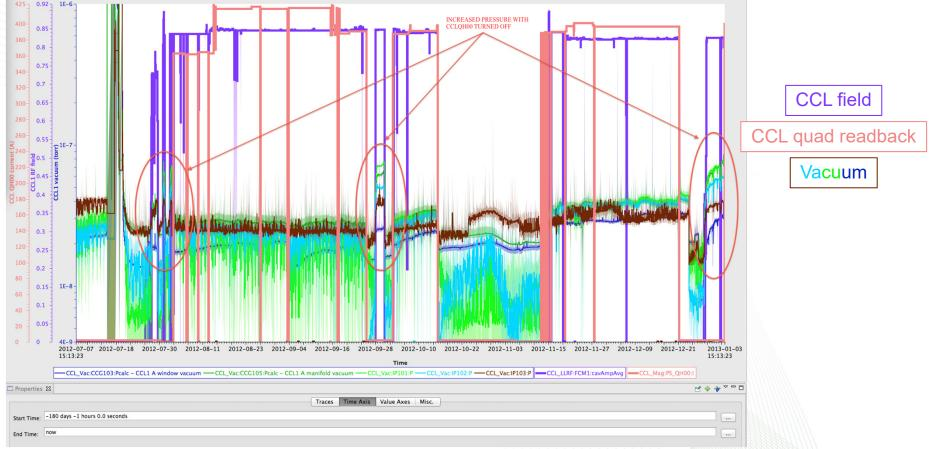
Without quads on the field emitted electrons heat up secondary equipment and cause contamination OAK RIDGE National Laboratory
