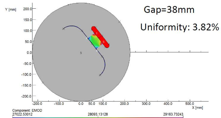
Simultaneous injection in H and V planes using **tilted** septum
