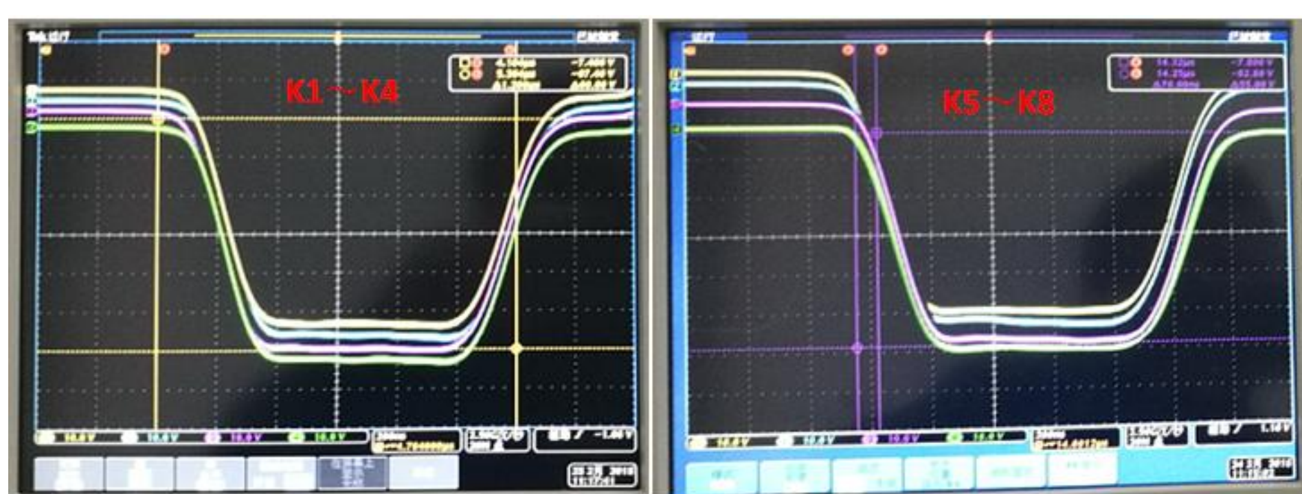
Fig. 3: Current curves of eight kickers.
