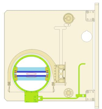
Figure 1: Wire Monitor MHP56Y (front, not all parts shown) and MHP55X (rear side, not visible) with 4-strip SEM MHB28 (green, foil strips blue) inserted and clamped to the base plate.  $2\sigma$  beam contours are indicated for regular (full red) and irregular (dotted red) beam. Beam comes out of drawing plane.
