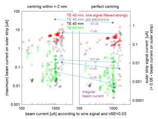
Figure 4: Maximum beam current passing one of the outer strips. The corresponding strip signal currents are estimated on the basis of the average secondary emission yield of  $n_{\rm SE} = 0.030$  deduced for the surface of the two 48  $\mu$ m Molybdenum wires of the wire monitor. The five examples from Fig. 3 are marked in blue.
