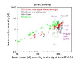
Figure 6: Maximum beam current passing one of the inner strips at centred beam. It is mainly given by current and vertical size of the regular beam.
