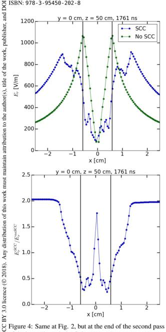
Figure 4: Same at Fig. 2, but at the end of the second pass of the beam through the Column. the terms of the
