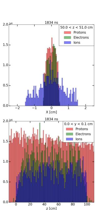
Figure 3: Distribution along x for the beam (red), electrons (green), and ions (blue) at the center of the Electron Column in z just before the beam would reenter the Column for a second pass - top. Note the beam distribution plotted is for the last time step that the beam is in the Column, for reference. Bottom - same as the top, but plotted along z at the center of the Column in y. The bin widths correspond to the simulation grid spacing.
