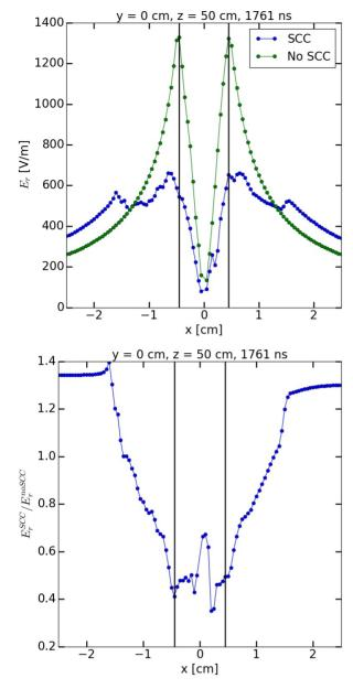
Figure 2: Radial electric field along x in the center of the column in y and z for beam alone (green) and with spacecharge compensation (blue) at the end of the first pass of the beam through the Electron Column - top. Ratio of the two electric fields from the top plot - bottom. The vertical lines in both plots denote the boundary of the beam.
