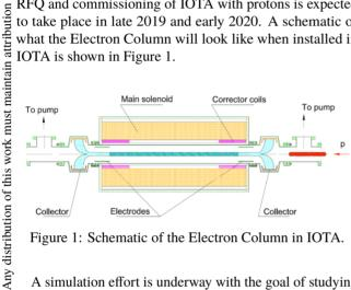
Figure 1: Schematic of the Electron Column in IOTA.
