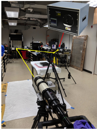
Figure 7: Using the blackbody source for calibration.
