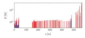
Figure 9: Power loss (per element) at 100% (red), 99% (blue) and 95% (green) confidence levels along the ESS LINAC.
