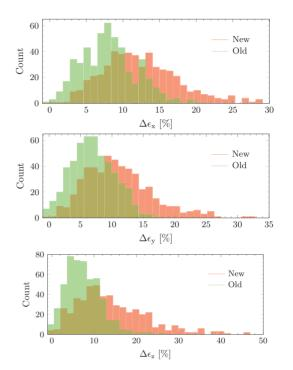
Figure 6: From top to bottom: Additional RMS emittance growth in the horizontal,  $\Delta \epsilon_x$ , vertical,  $\Delta \epsilon_y$ , and longitudinal,  $\Delta \epsilon_z$ , plane at the end of the high- $\beta$  cavities. The red color indicates that the accelerating field into the DTL is calculated solving the Maxwell equations (new method) while the green color indicates that E<sub>0</sub>, within the DTL, is modeled as a random variable uniformly distributed within its tolerance (1%).
