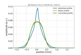
Figure 11: A case with particularly distorted profile. Original beam distribution is generalized gaussian with  $\beta = 3$ . ANN corrects the profile very accurately.
