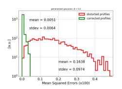
Figure 10: MSD for profiles with generalized gaussian distribution with  $\beta = 3$ : before and after correction.
