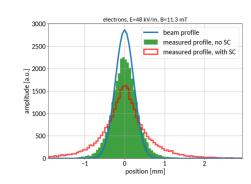
Figure 4: Simulated distortion of beam profile measured in LHC IPM.
