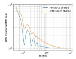
Figure 5: Dependency of the profile distortion on the IPM magnetic field.
