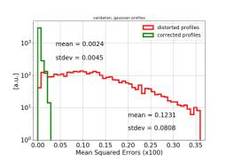
Figure 9: Mean Squared Deviation for gaussian profiles before and after correction.
