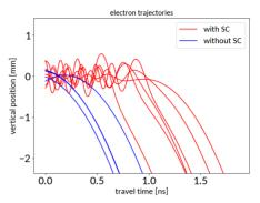
Figure 7: Simulated trajectories of the electrons. The vertical position as a function of time, zoomed to the first 1.5 ns after ionization.
