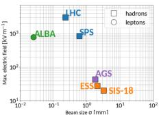
Figure 1: Comparison of typical maximum bunch electric field and beam size for various machines.
