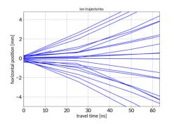
Figure 3: Examples of ion trajectories. The coordinate along the profile of positions are shown as a function of travel time.
