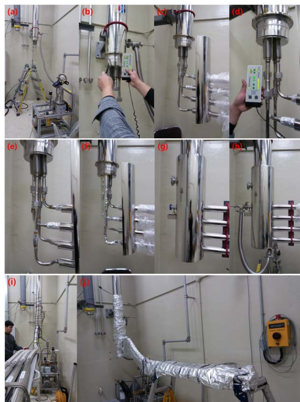
Figure 1: Fabrication process of liquid helium and liquid nitrogen transfer lines for cryomodules test from (a) through (f).
