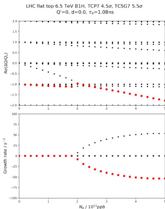
Figure 2: Complex Tune Shift as a Function of Intensity. Results for tighter collimators settings are showed, for a chromaticity of zero units.
