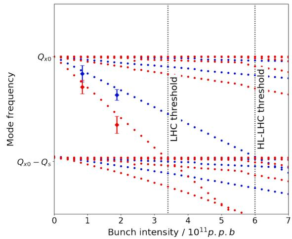
Figure 4: Measured (diamonds) and simulated (dots) tune-shifts as a function of intensity for the nominal LHC collimators settings (in red) and for the equivalent HL-LHC impedance collimators settings (in blue). The plane showed is B1H, for an unnormalized chromaticity of +5, without damper.
