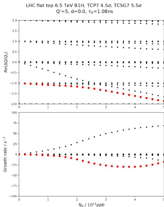
Figure 3: Complex Tune Shift as a Function of Intensity. Results for tighter collimators settings are showed. The unnormalized chromaticity is now 5 units.
