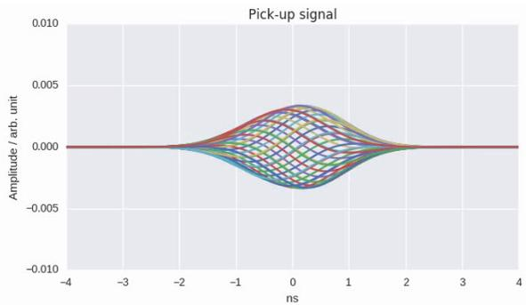
Figure 5: Intra-bunch motion in the mode coupling regime, with a positive chromaticity and above transition. The signal is reconstructed from the eigenvectors output of DELPHI. The horizontal axis is the bunch length.
