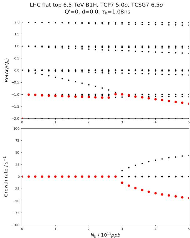
Figure 1: Complex Tune Shift as a Function of Intensity. The nominal LHC collimators configuration is showed, for a chromaticity of zero units.
