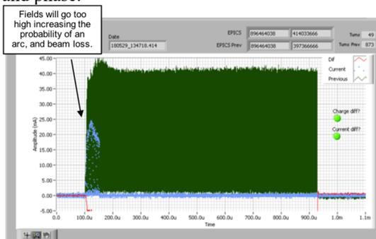
Figure 6: Example of an ion source high voltage arc. The green pulse is a nominal pulse and the blue is the beam current during an ion source malfunction.
