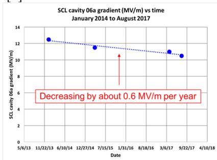
Figure 4: The plot above shows the need to decrease SCL cavity 06a gradient over time. The reduction is about 0.6 MV/m per year.
