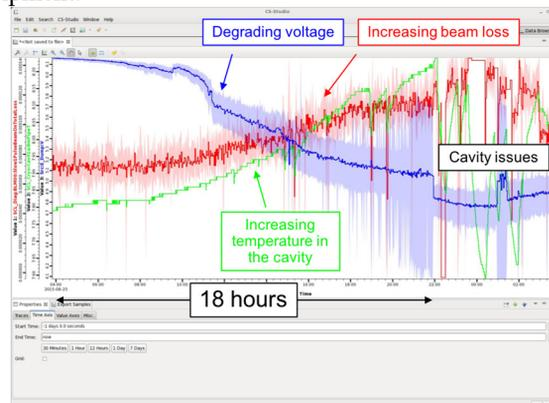
Figure 7: The plot above shows the degrading ion source voltage (blue), increasing beam loss (red), and the increasing beam pipe temperature (green) in an SCL cavity. After ~18 hours of increasing beam loss SCL cavity issues developed requiring reduced gradient.
