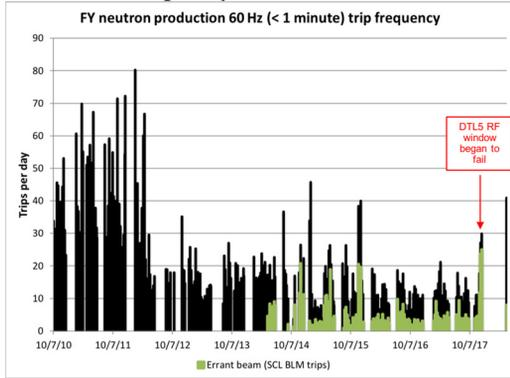
Figure 12: The plot above shows the reduction in short fault frequency dominated by errant beam faults.
