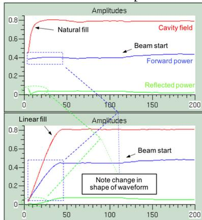
Figure 8: Top shows the natural cavity fill. The bottom shows the adjustment to the linear forward power fill.
