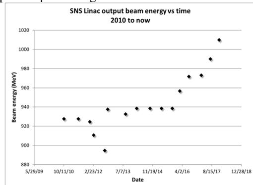
Figure 14: The plot above shows the linac beam output energy versus time. Since 2016 plasma processing has significantly increased the beam energy.
