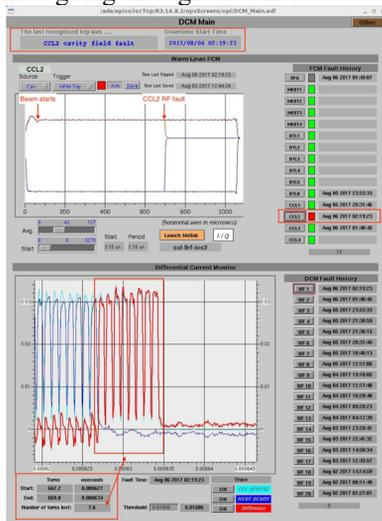
Figure 13: The snapshot above is an example fault detection by the SCL DCM system.
