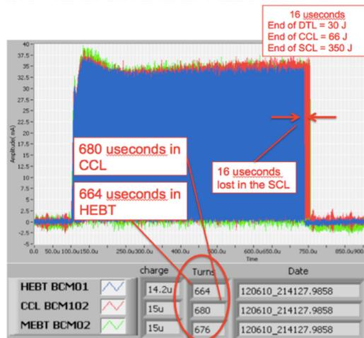
Figure 5: The above figure shows the BCM system used to verify that the MPS was turning off the beam at the design time of 20 microseconds.
