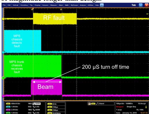
Figure 3: Scope snapshot showing delays of 200 microseconds during the MPS issues found in 2009.
