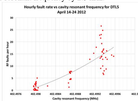
Figure 9: Reduction in fault rate by lowering the DTL5 cavity resonant frequency.
