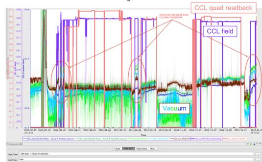
Figure 10: The plot above shows elevated vacuum pressures when quads powered off with RF on.
