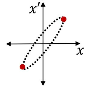
Linear mapping of the measured rms beam size onto the initial phase space.
