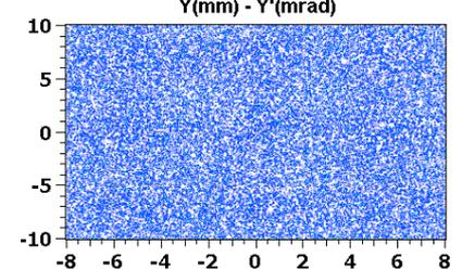
Transverse phase space plots of the test beam
