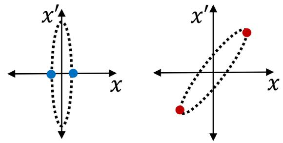
Linear mapping of the measured rms beam size onto the initial phase space.
