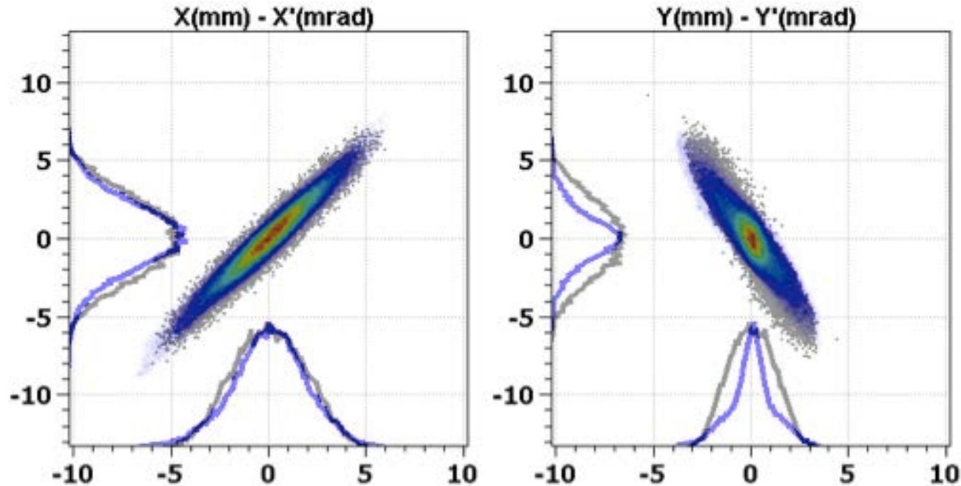
Comparison of phase space plots of the expected beam (grayscale) and measured at 50 MeV (colour scale) after the DTL.
