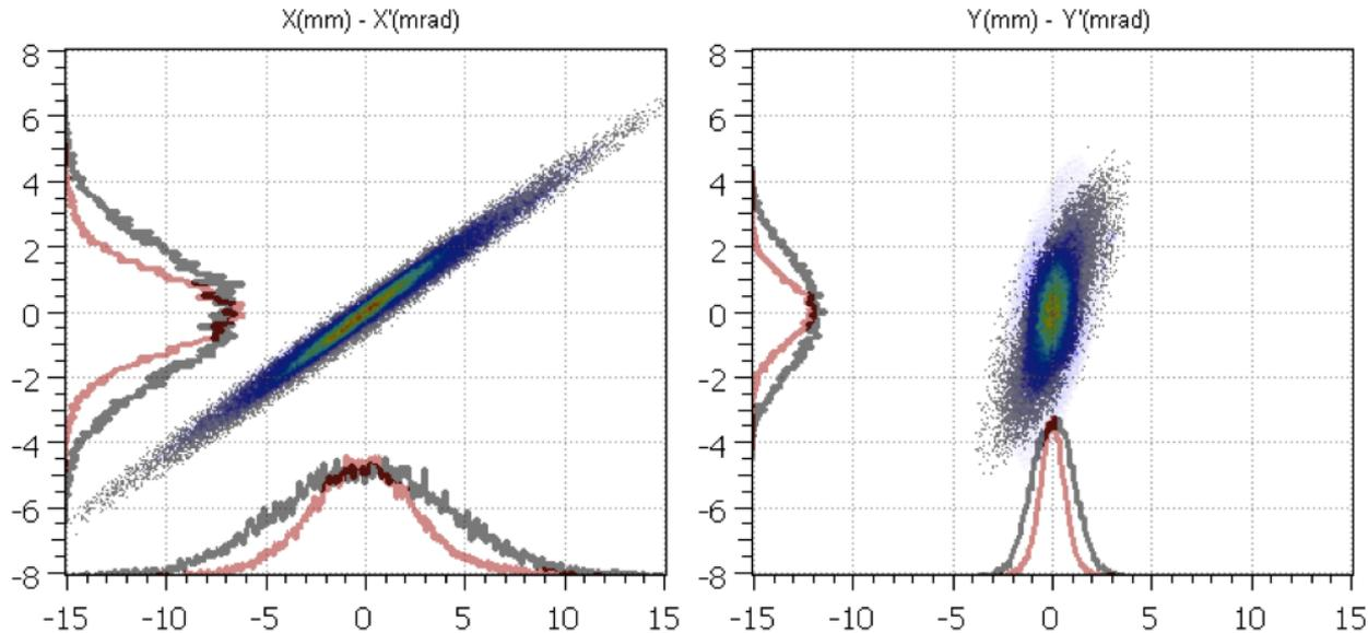
Comparison of the phase space plots of the expected (grayscale) and measured (colour scale) beams at 50 MeV.
