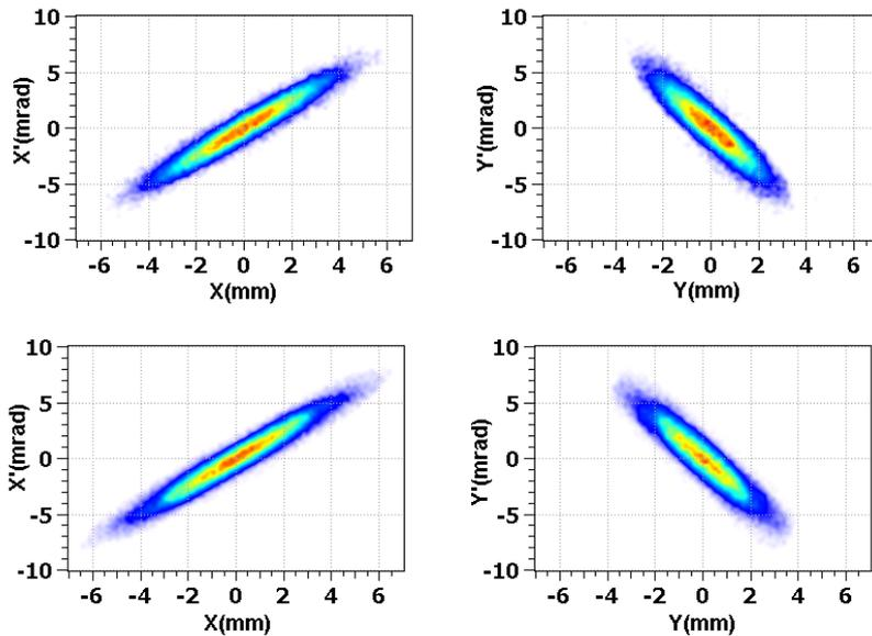
Transverse phase space plots of the reference beam (top row) and the reconstructed beam (bottom row).
