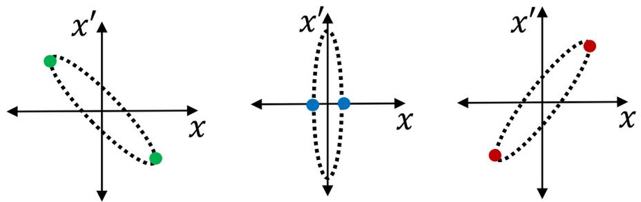
Linear mapping of the measured rms beam size onto the initial phase space.
