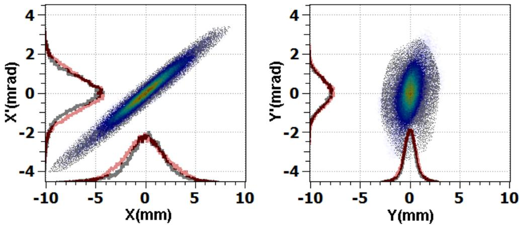
Comparison of the phase space plots of the beams measured at 80MeV (grayscale) and measured at 50 MeV then tracked to 80MeV (colour scale).
