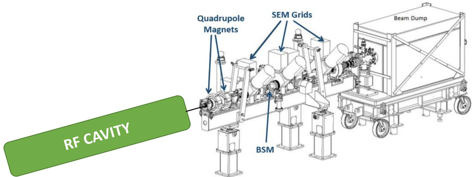
Both forward method and hybrid phase space tomography can be applied to the longitudinal phase space reconstruction where the phase and/or amplitude of an RF cavity is varied and the phase or momentum profile is measured downstream. In the case of Linac4, phase spread was measured by a BSM.
