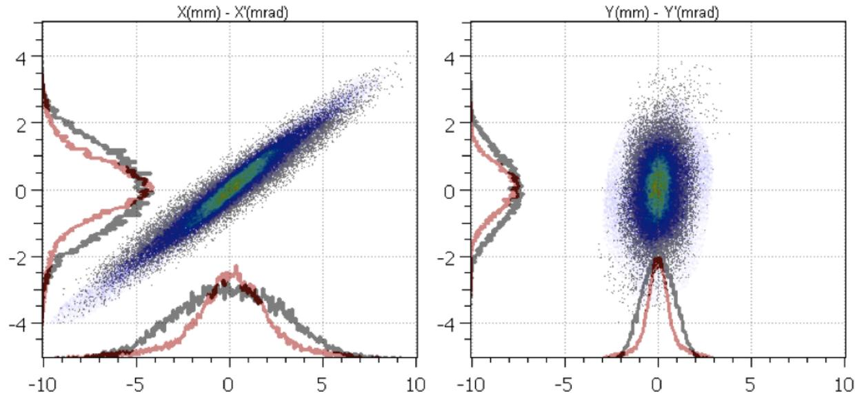
Comparison of the phase space plots of the expected (grayscale) and measured (colour scale) beams at 80 MeV.
