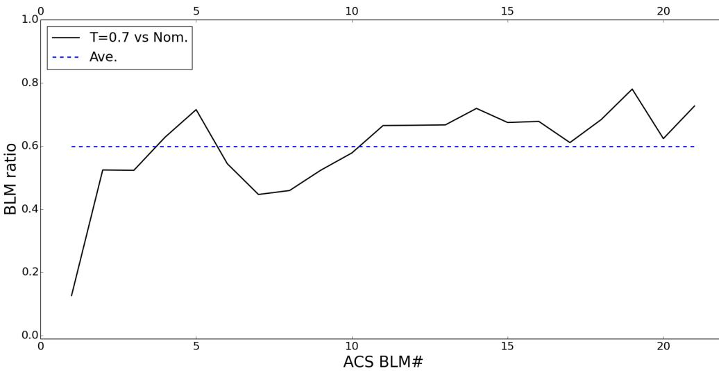
Beam loss:  $T=0.7$ , -40% reduction of beam loss vs. nominal.
