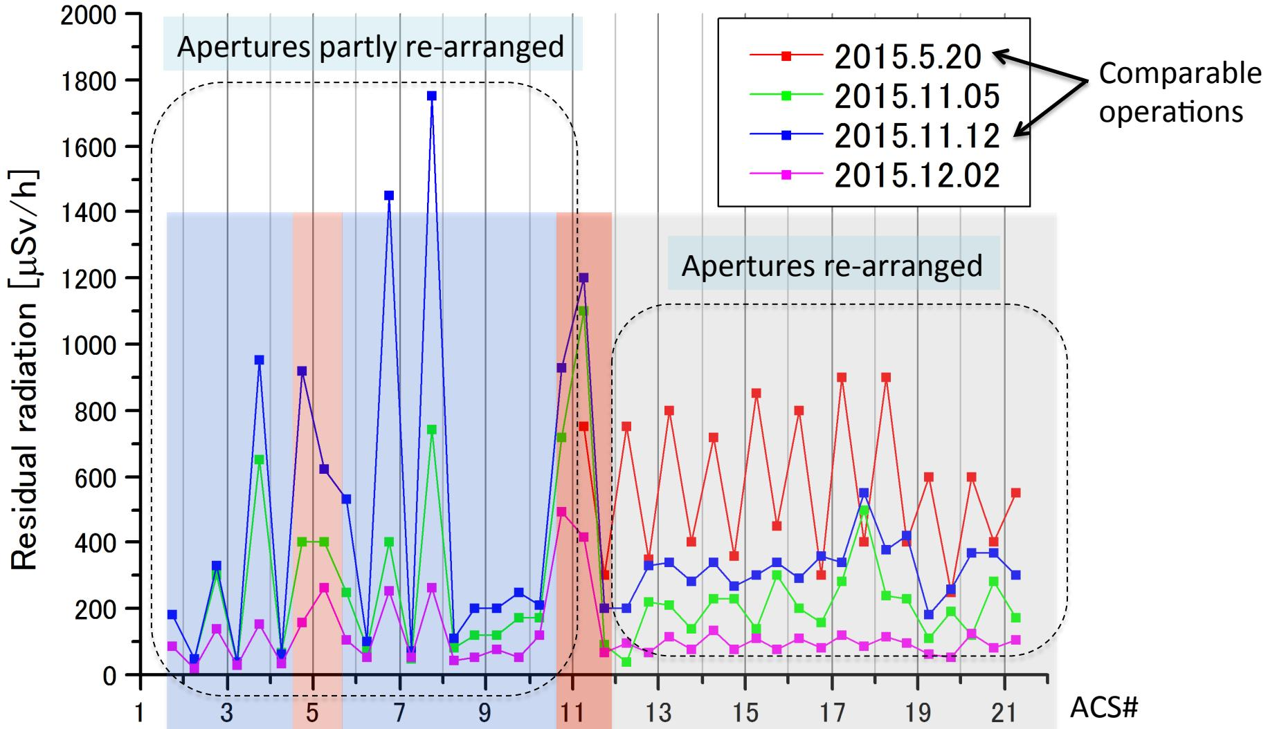
With linac 30mA, RCS 300kW user operation (red & blue), residue dose (surface) reach 1mSv/h level
