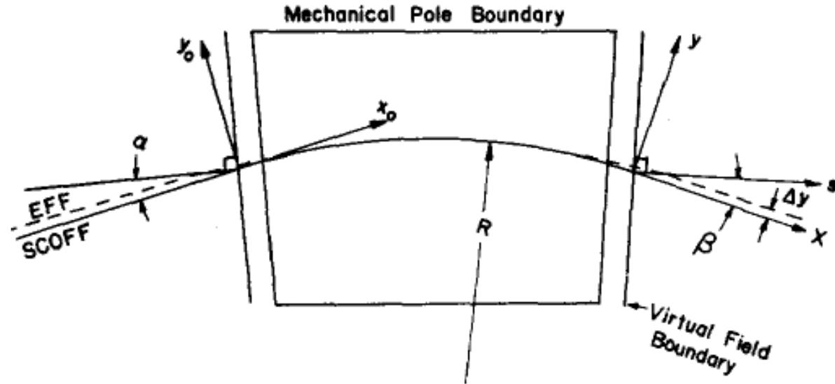
Midplane field of the 45° dipole in the first 180 bender with orbits
