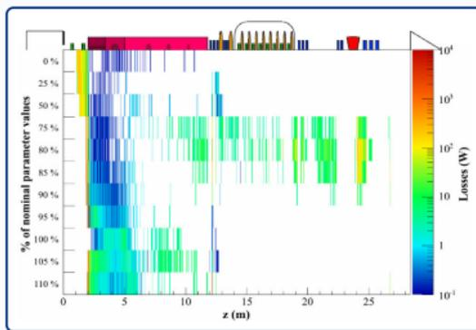
*Power lost in case of LEBT and RFQ failure*
