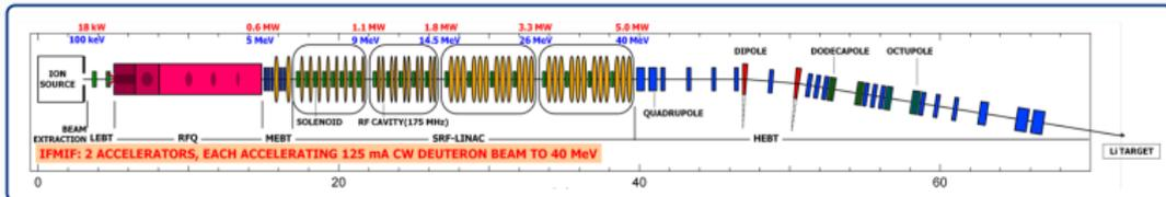
**IFMIF Accelerator: 125 mA/40 MeV D<sup>+</sup> beam – 5 MW**
