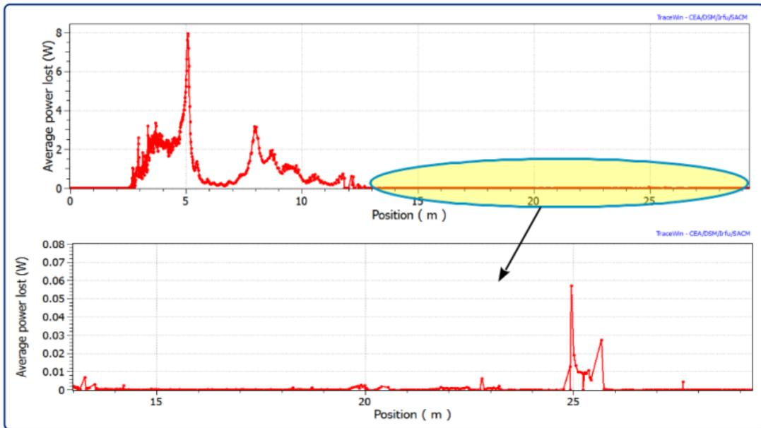
**Beam losses in Watt through the accelerator**
