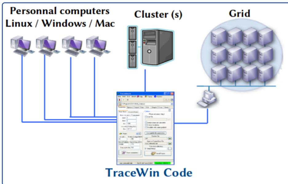
**Distributed calculations using the TraceWin code**
