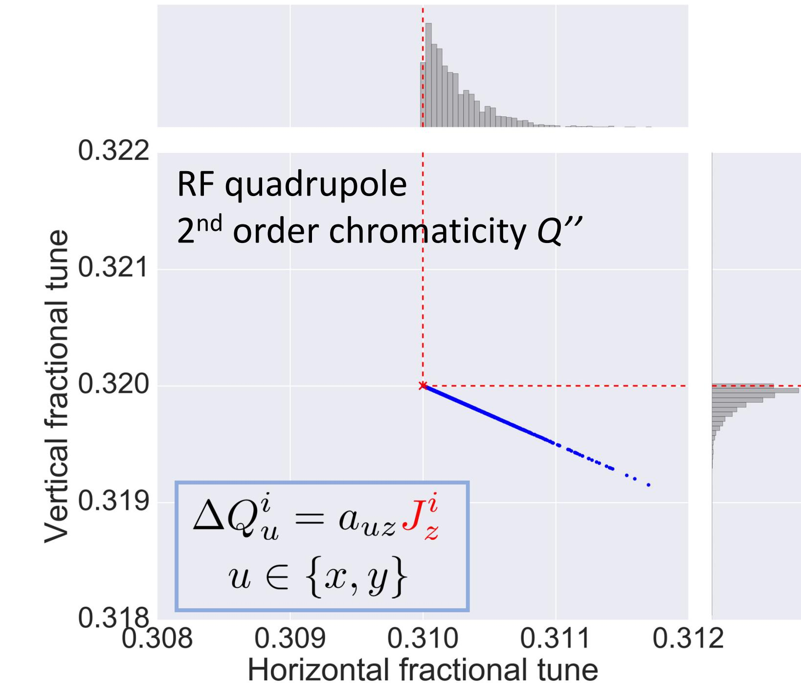
**Detuning strength is directly affected by the smaller transverse beam size (action spread).**
