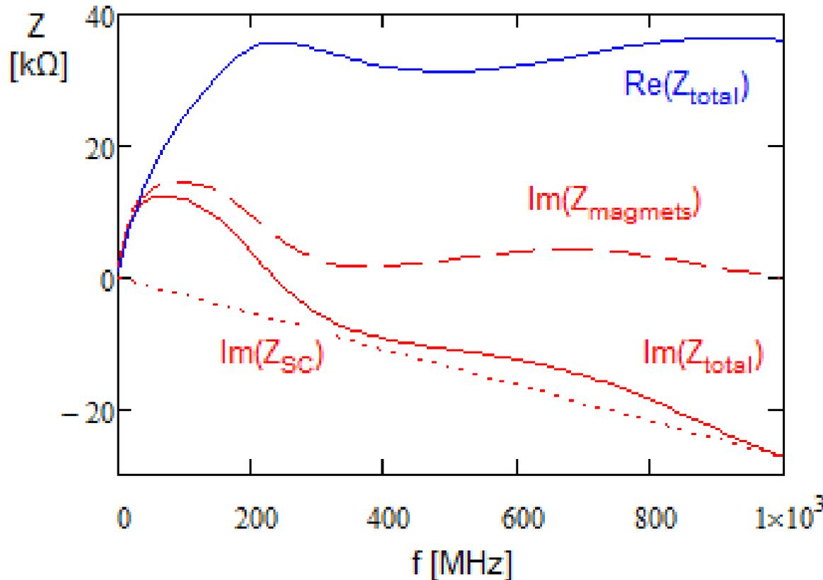
*Total  $Z_{||}$  for Booster at transition. The value is tuned to the beam-based measurements*
