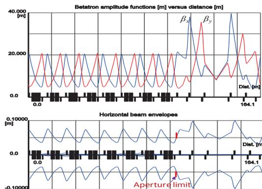
Twiss parameters and horizontal beam envelope for one super-period at the BRing
