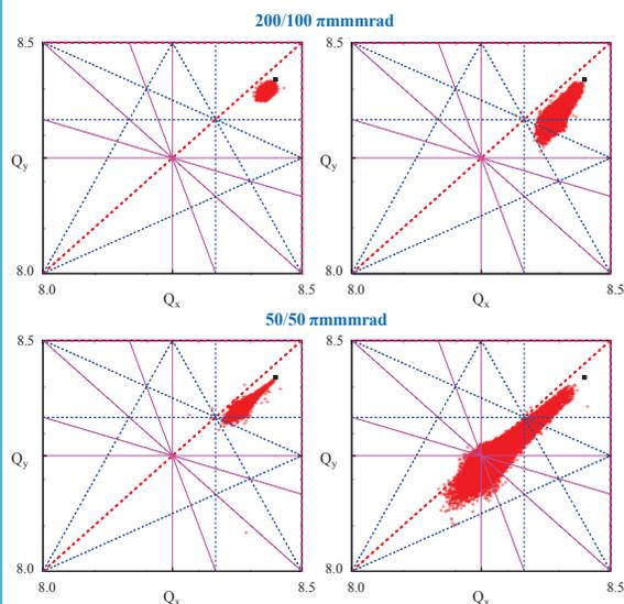
a). Crossing resonance stop-bands for bunched beam while coasting not.
