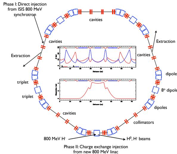
Figure 1: ISIS upgrade RCS showing lattice and optical parameters. Injection in the first phase would be directly from the present 800 MeV RCS, with a new system of  $H^-$  painting from a new linac in Phase II.
